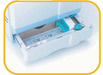
Card Hopper holds up to 300 cards (0.76mm)
