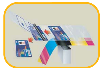
Re-transfer printing process First, the card design is printed in colour onto the reverse of the clear re-transfer film. The printed film is then released from its carrier and applied to either side of a plastic card.
